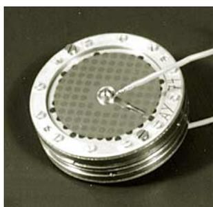
A switch located on the microphone head permits changing the low frequency attenuation to become effective at 100 Hz for proximity compensation. The EF 86 tube operates as triode in an anode amplifier configuration into an output transformer with separate feedback windings. The output transformer's special construction helps to eliminate hum and allows internal impedance matching with the following preamplifier.
