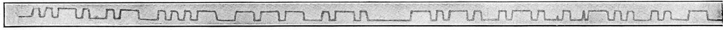
HOW SHORT WAVE HIGH POWER— A section of tape, part of a message received at the Broad Street offices of the Radio Corporation of America from station SAQ at Gothenburg, Sweden. The message reads: "Favor creditbank Oslo 2." The effects of static can be seen in several places appearing as a sharp pointed mark much narrower
