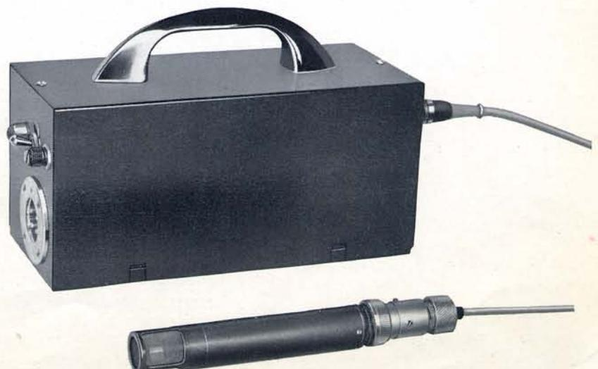
In the design of the amplifier and mains supply unit, particular care has been taken to eliminate sources of noise. A special valve, which can tolerate an extremely high grid resistance without significant increase in noise level, is used in the first stage of amplification. This is followed by a transistor buffer stage that increases amplification and greatly eases matching problems.
