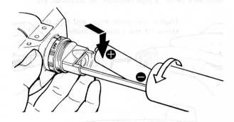
Close the compartment by turning the sleeve clockwise. Be sure to close the sleeve firmly, otherwise malfunction or noise may occur due to the loose fit.
