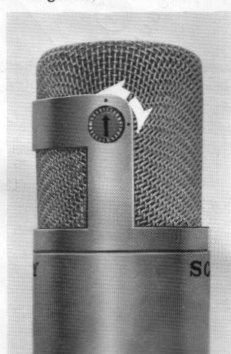
The capsule is locked as the fingers are released. The arrow mark on the button shows the direction of the capsule. Direct the arrow mark toward the sound source. The arrow mark is set to 45 degrees position when the microphone is mounted on the boom-stand. The microphone can be rotated around the axis of the unit which gives an optimum pick-up for sounds coming from many directions.
