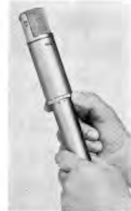
Figure-5 C-55 FET condenser microphone, turning operation, main switch
