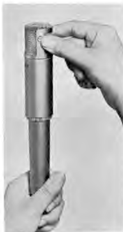
Figure-14 C-55 FET condenser microphone, turning capsule operation
