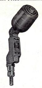
Smart, modern appearance, excellent fre-quency response and flexibility of operation. Frequency response: 40-8,000 c.p.s., unusually flat through lower and middle register rising 5 DB on upper frequencies for added crispness of speech. Output: —54 db (below 6 millowatts/10 dyne/cm²). Full equipment includes "on-and-off" switch, tilting head for directional or non-directional operation, 20' cable and cable connector. Available in all impedances (low impedance, balanced to ground)
