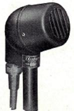
A leader in the lowest price field. De-pendable quality, maximum durability and modern appearance. Response is desirable for all types of sound work, recording and communication. Microphone has a fixed 22° tilt. There has been no compressise in design or choice of materials. Frequency response: 47-7,500 c.p.s. 8' cable. Output: —56 db (below 6 milliwatts/10 dynes/cm²). Low impedances not balanced to ground,
