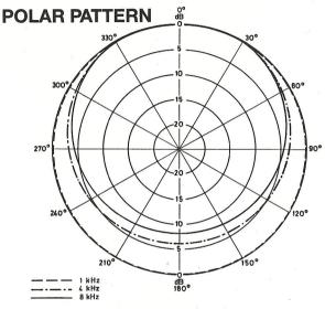
This polar pattern and frequency response curve correspond to typical machine run specifications from a standard M 58.
