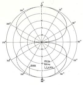
This polar pattern and frequency response curve correspond to typical machine run specifications from a standard M 130.
